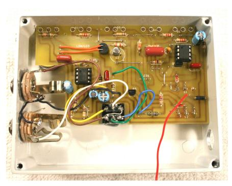
Since all of the wiring is done except for the power jack, you can now do a full-function test. Connect your guitar and amplifier, and temporarily connect the battery. The negative lead goes to the common ground at the sleeves of the jacks. An alligator clip lead will help in setting this up. Bring up the Level control some and raise the Bias and Intensity. Check out the operation of the stomp switch. Got the effect? Controls work? Stomp switch works OK?
