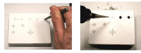
In a similar way, fasten the templates and drill the holes for the DC power jack and the input and output jacks.
