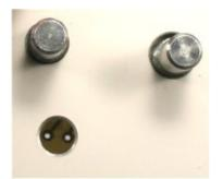
Once the board goes into the case smoothly, slip the washers and nuts onto the pots and switch and finger-tighten. When tightening the nuts, be sure that none of the components is being pulled out-of-true. If you notice any of that, disassemble and go back to work with the file
