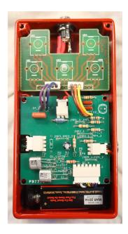
Plug in your gear and connect a battery. Does the in-use LED light up? Click the stomp switch if not. If the LED does not light, you have at least one problem. **Stop** here and go to the section on troubleshooting. If the LED lights, see if the controls work. The tone should be Rangemaster-ish trebly at the counter-clockwise side and more full-spectrum at full clockwise. Level should give you good control of volume. If they work...
