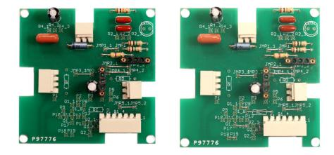
Add the five jumpers that configure the connections for the build.
