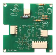
In designing a PC board, it is common to use short pieces of bare wire, called "jumpers" to avoid the expense of making a board with copper traces on both sides. Take one of the scraps of wire that (I hope!) you saved from the resistors, and bend it to exactly span the holes marked JMP1\_1 and JMP1\_2. Hold it in place with tweezers and solder. The pic on the right shows the locations of all five jumpers; form the rest and solder in place.
