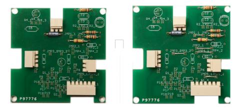
Install the poly film capacitors C2, C3 and C5. It is easy to confuse C2 and C3 because their lead spacing is the same, so pay close attention to the codes. C3 is 153, or .015 mf. They are not polarized. Then install radial electrolytic capacitors C1 and C4. These are polarized, so be sure to align them as shown in the right-hand pic. The band on C1 faces the bottom of the board, and the band on C4 faces the top.
